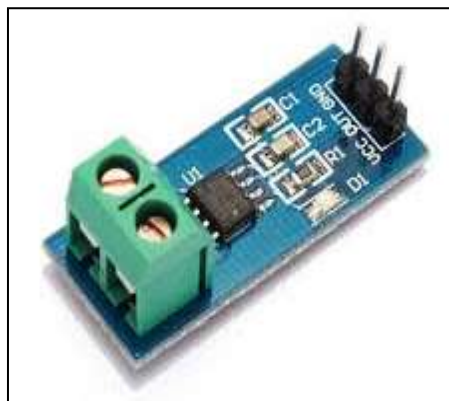
Figure 4: ACS712 Current Sensor
